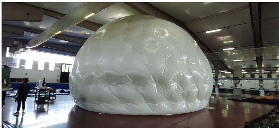
Figure 14: Test inflation of the finalised translucent envelope (source: Canobbio)
