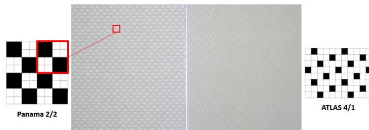
Figure 4: characteristics of ATLAS weave
