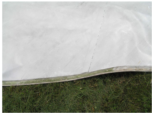
Figure 2b: PVC/PET fabric after 5 years
