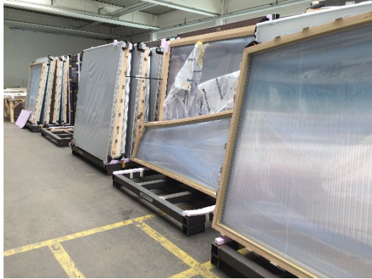
Figure 15: ETFE-modules completed and released, ©Taiyo Europe
