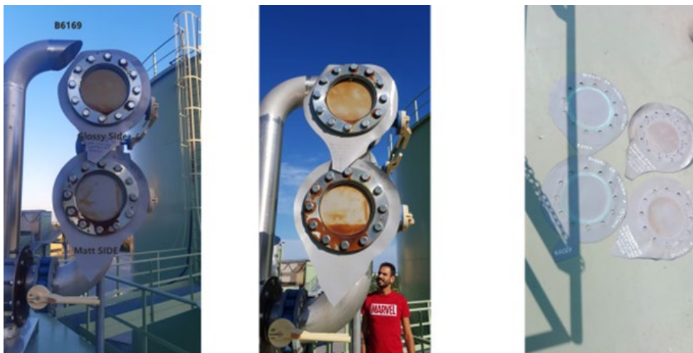
Figure 2: Field test exposing the gas membrane to raw biogases before conducting material analyses.
