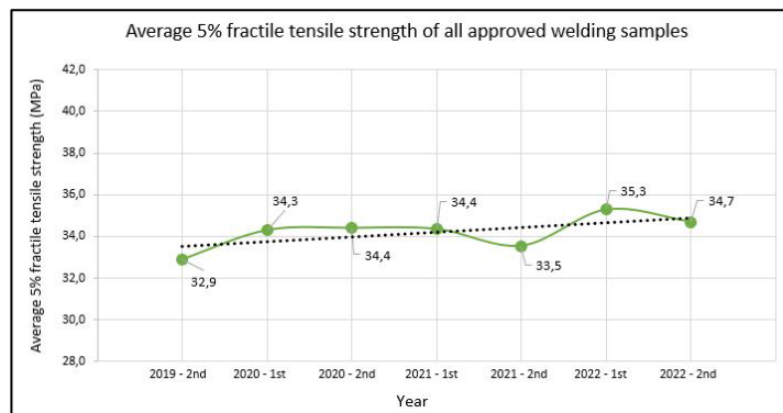
Figure 6: Average 5% fractile value of the tensile strength of all approved samples from 2 nd half year 2019 until 2 nd half year 2022 (7 inspection periods)
