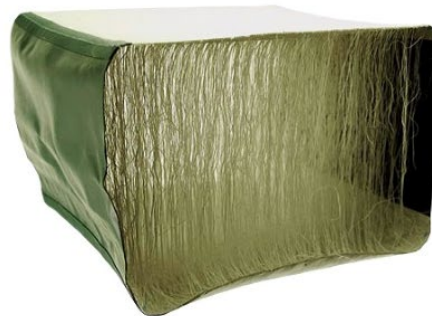
Figure 3: Cut-views of double-wall fabric with drop cords.
