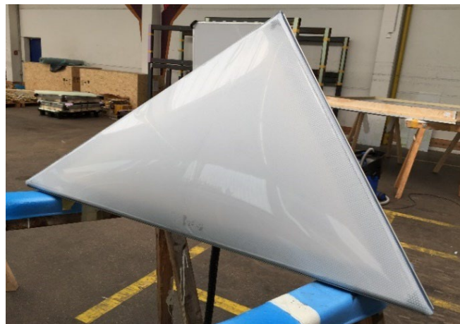
Figure 7: White ETFE-foil element mounted on a timber frame and tested with an internal overpressure, ©Taiyo Europe
