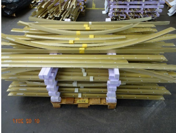
Figure 8: Clamping profiles anodized in a golden tone, straight, pre-bended and pre-twisted, ©Taiyo Europe
