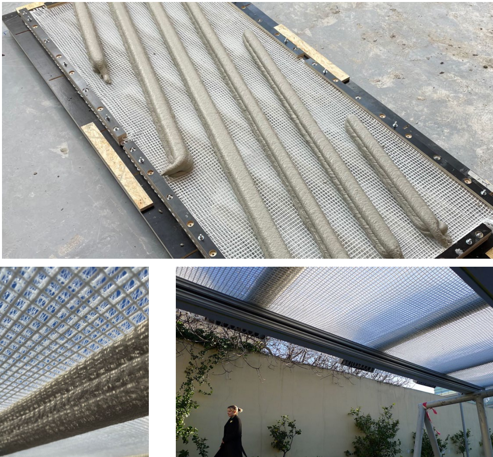
Figure 11: Upscaling, ceiling and wall elements from 3D textiles combined with 3D concrete printing © FRAUAS
