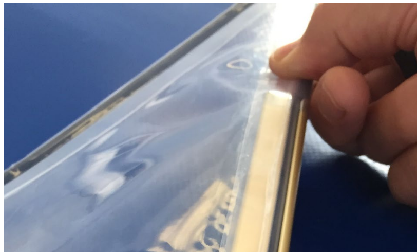
Figure 5: 1:1 test sample of a sharp ETFE-foil-corner produced by Diaferia, ©Taiyo Europe
