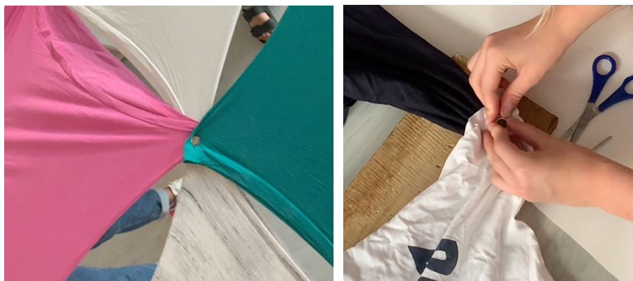
Figure 4: Connection of wasted t-shirts using grommets to create a large membrane for urban shading system.
