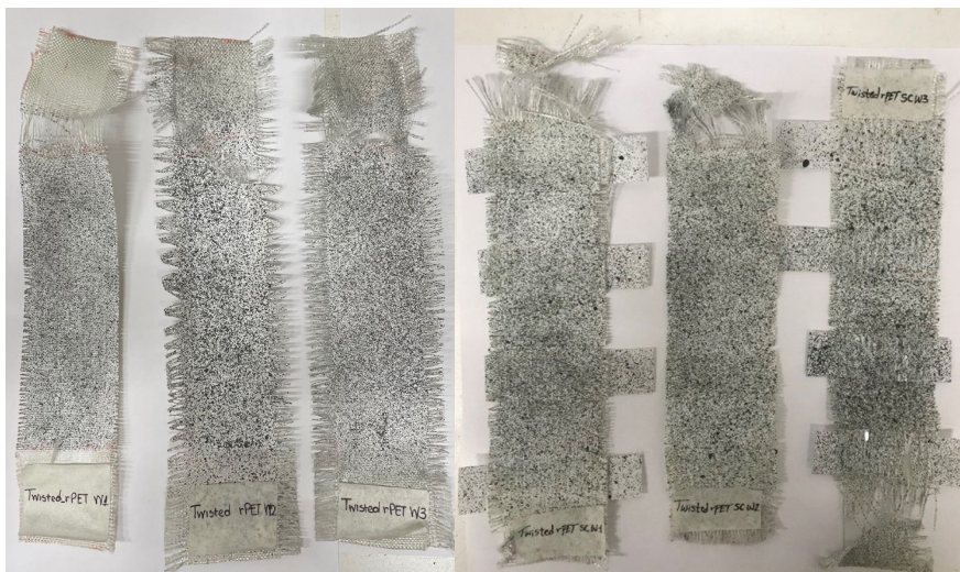
Figure 5. Suntex V2 Specimens after testing to failure. Regular specimens labelled “Twisted rPET W1-3” are referred to as “Suntex V2 W1-3” in this paper, and Solar Film specimens labelled “Twisted rPET SC W1-3” are referred to as “Suntex V2 SF W1-3” in this paper.
